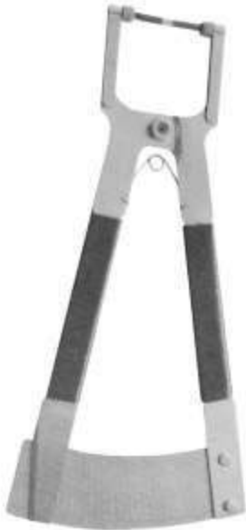
MSI-2183-00 Wide Throat Lens thickness Gauge Accomodates Lens Blanks of over 90mm Diameter & 22mm in thickness 47mm Throat Depth, 0.1 mm Graduations overall Length 9.3/4"
